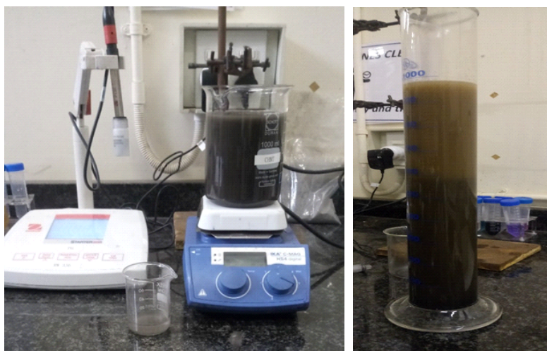
Fig. 3. Slurry preparation setup and settling test setup
